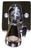
H-08 institutional shower head, brass, ball joint, adjustable spray, vandal-resistant screws, 2.5 GPM (9.5 l/min)
