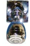
H-15 Low Flow institutional shower head, brass ball joint, vandal resistant screws, 1.5 GPM (5.7 l/min)
