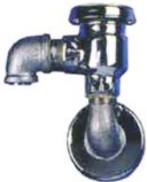
LVB elevated vacuum breaker, chrome-plated, 1/2" with hose connection on outlet
