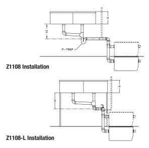
Maximum distance in inches from bottom of sink to centerline of flow control fitting inlet (D).
