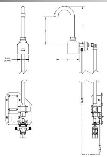
(2) 18" braided stainless steel supply lines included DC models powered with (4) 1.5V AA batteries (included)
