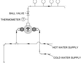
CIRCULATE HOT WATER FROM END OF LINE BACK TO TANK
