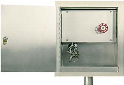
OR-1775 Manual Station for Dialysis Applications The water outlet assembly includes an atmospheric vacuum breaker, volume control/shutoff and stainless steel quick coupler with dust cover. The unit is mounted in a stainless steel recessed cabinet with drain, door with cylinder lock, and panel with vandal resistant screws.
