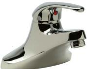
Engineering Specifications: Zurn AquaSpec<sup>®</sup> Single Control Faucet Z81000 Polished chrome plated cast brass 4" [102mm] centerset single control lavatory faucet, a ceramic disc cartridge and a temperature limit stop. Unit is furnished with 2.2 GPM [8.3 L] aerator (complying with ANSI A112.18.1M Standard for flow), an ADA compliant lever handle, mounting hardware, 1/2" NPSM coupling nuts for standard lavatory risers, and pop-up hole plugged.
