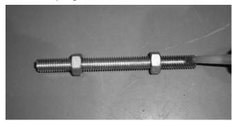
Thread the worm stem assembly until seated fully and then thread the plunger assembly to match the length of the old hydrant stem assembly. (Remove excess thread locker.)
