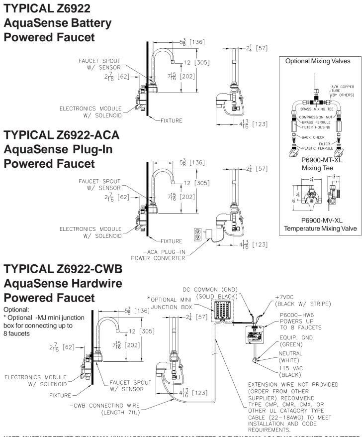
NOTE: MUST USE EITHER ZURN P6000-HW6 HARDWIRE POWER CONVERTER OR ZURN P6000-ACA PLUG-IN POWER CONVERTER TO ENSURE PROPER OPERATION. USING A POWER CONVERTER OTHER THAN ZURN MAY RESULT IN OPERATION MALFUNCTION OR UNIT FAILURE.
