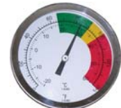
2122 FOR TEPID APPLICATIONS range: 0-140°F, -20-60°C, 15/16" bulb, special 4 color, 3-1/2" dial, bimetal type
