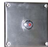
LV477B-3 metering valve, concealed, pushbutton activation, fixed cycle, 30 seconds, inlet stop, exposed parts chrome-plated, 1/2" IPS connections
