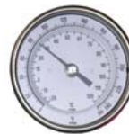
37C20A range: 20-240°F, 5-115°C, 1.12" bulb, 3-1/2" black dial, bimetal type
