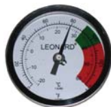
37C30A range: 0-140°F, -20-60°C, 15/16" bulb, 3 color, 3-1/2" dial, bimetal type
