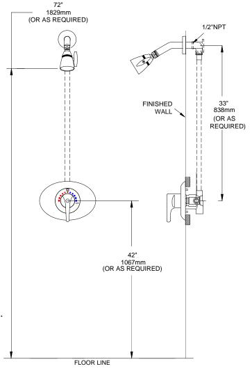
All Leonard Model 7600 Thermostatic Shower Valves have limitations. Please keep in mind that per the ASSE 1016-2011 Performance Standard, Harmonized along with ASME and CSA, it dictates inlet conditions of equal pressures, 45 PSI on both Hot and Cold Inlets, in addition to a Hot supply temperature range of 140 deg F- 180 deg F. Significant deviations from those conditions stated above will alter performance expectations.
