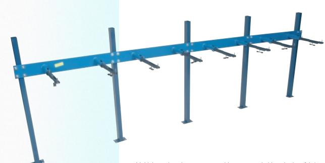
Multiple station plate system provides an extended length plate fabricated with exact center-to-center locations to accommodate a bank of multiple lavatories. Custom-length plates are specific to job requirements and are provided with welded steel sleeves. Uprights and arms are provided loose with boxed mounting hardware. Ideally suited for pre-fabricated applications.
