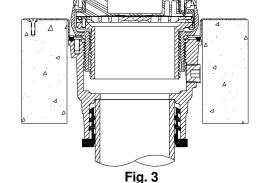
3B. If installing a cleanout, ensure cleanout plug is installed in the cleanout body.
