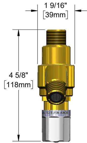
Locking Adjustment Knob Prevents Water from Exceeding Customer's Maximum Temperature Set Point.
