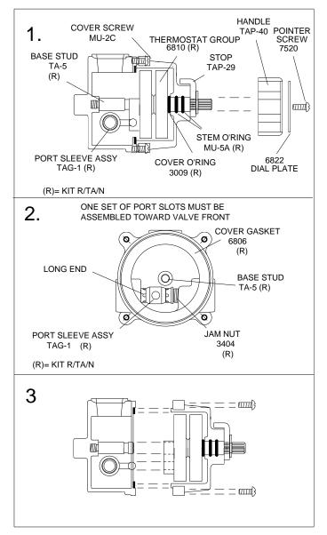
After installation, adjustment, cleaning, always check the temperature of the valve when turned to full **HOT** per the warning on the front page, using a thermometer. Also check and if necessary adjust the temperature of the hot water source. **EXCESSIVELY HOT WATER (OVER 110°F) IS DANGEROUS AND MAY CAUSE SCALDING!!**
