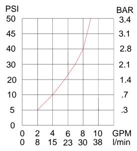
**CAUTION!** All thermostatic water mixing valves have limitations. They will not provide the desired accuracy outside their flow capacity range. Consult the capacity chart and **DO NOT OVERSIZE.** Flow must not be greater or less than as shown below.
