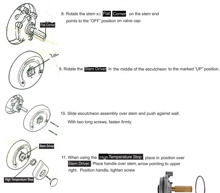
NOTE: When placing the High Temperature Stop over the Stem Driver, move the Stop left for hot and right for cold, to set a limit for the desired water
