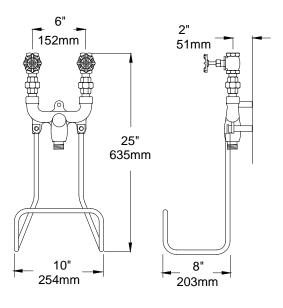
**IMPORTANT!** The prevailing steam (or hot water) pressure must be slightly lower than the cold water pressure.
