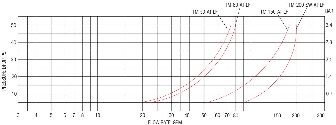
**CAUTION:** All thermostatic water mixing valves have limitations. They will not provide the desired accuracy outside of their flow capacity range. Consult the above chart and graph and make certain minimum flow is greater than as shown above.
