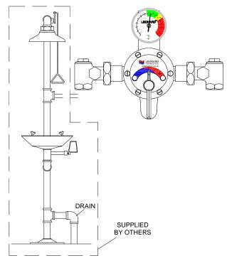
This product is certified to meet Low Lead requirements of wetted surface area containing less than 0.25% lead by weight
