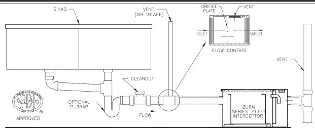
Zurn Grease Interceptors Z1171 consist of a interceptor rated at ( ) gpm and a properly sized flow control fitting. **INSTALLATION**
