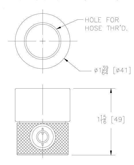
**ENGINEERING SPECIFICATION:** Z1399-HG Brass hose bibb lock with key operated lock/un-lock feature for 3/4 [19] hose thread connection.
