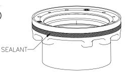
**Step 9** Replace the strainer B onto the frame D and secure strainer with the three #8-32 x 1/4 flat head strainer screws. (A)
