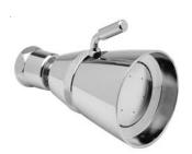
**ENGINEERING SPECIFICATIONS:** Self-cleaning brass shower head with hard chrome plated finish, brass chrome plated ball joint connector, maximum flow rate 1.25 GPM at 80 PSI, 1/2" NPT female threaded inlet, body width spray pattern adjusts from needle shower to heavy wash.
