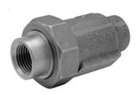
**ENGINEERING SPECIFICATIONS:** Z7000-SC In-line spring loaded dual check valves with 1/2" FC (copper) "union" inlet connection x 1/2" FC outlet connection. Supplied as a pair, assemblies are designed for installation on hot and cold inlet connections of ZURN pressure balanced shower valves where positive cross-connection (ie: medical installations, spas & jacuzzis) is required. Assemblies shall be installed with union connection facing outward to allow for maintenance.
