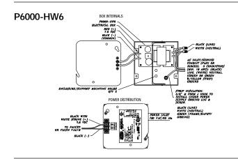
ENGINEERING SPECIFICATION: Zurn P6000-HW6 Hardwire Power Converter – Hardwire power converter to power up to 8 Zurn sensor urinal/closet flush valves or up to 8 hardwired Zurn sensor faucets. The P6000-HW6 is mounted on a 4-11/16" x 4-11/16" cover plate that mounts to a standard 4-11/16" x 4-11/16" electrical box (supplied by others).
