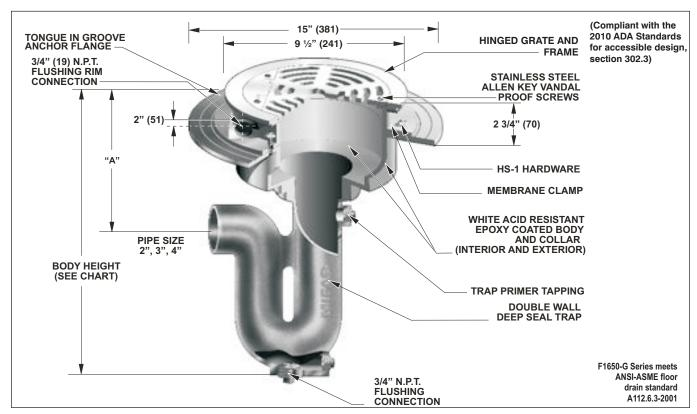
**Note:** See F1670 for water supply control box to be used with the flushing rim floor drain Use a vacuum breaker between the potable water supply and the connection to the flushing rim connection (by others).
