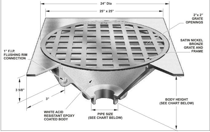
**Note:** See F1670 for water supply control box to be used with the flushing rim floor drain Use a vacuum breaker between the potable water supply and the connection to the flushing rim connection (by others).
