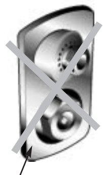
HYDRANT FACEPLATE IN INCORRECT VERTICAL POSITION
